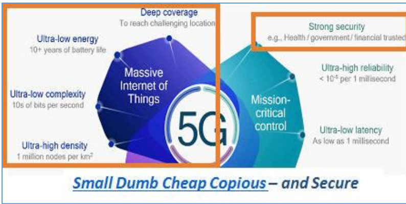
Fig. A. Left: Key Challenges to “Massive IoT”: Energy, Complexity, Density + Security. In incumbent offerings massive deployment - density, simplicity, low power, and remote hostile environments conflict high security, requiring processing power.
